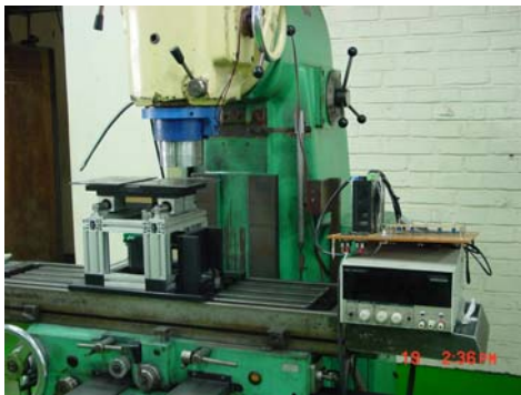
Fig.2 Vibration table and controller
